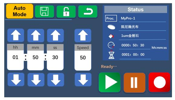
The running speed can be directly modified the device is working, and the running time needs to be "stopped" and then "started" again.
