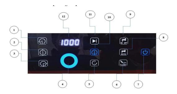
(1)(2)(3): Three gears preset revolving speed, press the button and running speed will be based on the saved values. In this mode, the revolving speed can not be adjusted.
