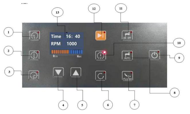
(1)(2)(3) : Three gears preset revolving speed, press the button and running speed will be based on the saved values. In this mode, the revolving speed can not be adjusted;
